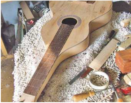
▲ Pic.27 Sand and scrape the guitar, removing any traces of glue squeeze-out
